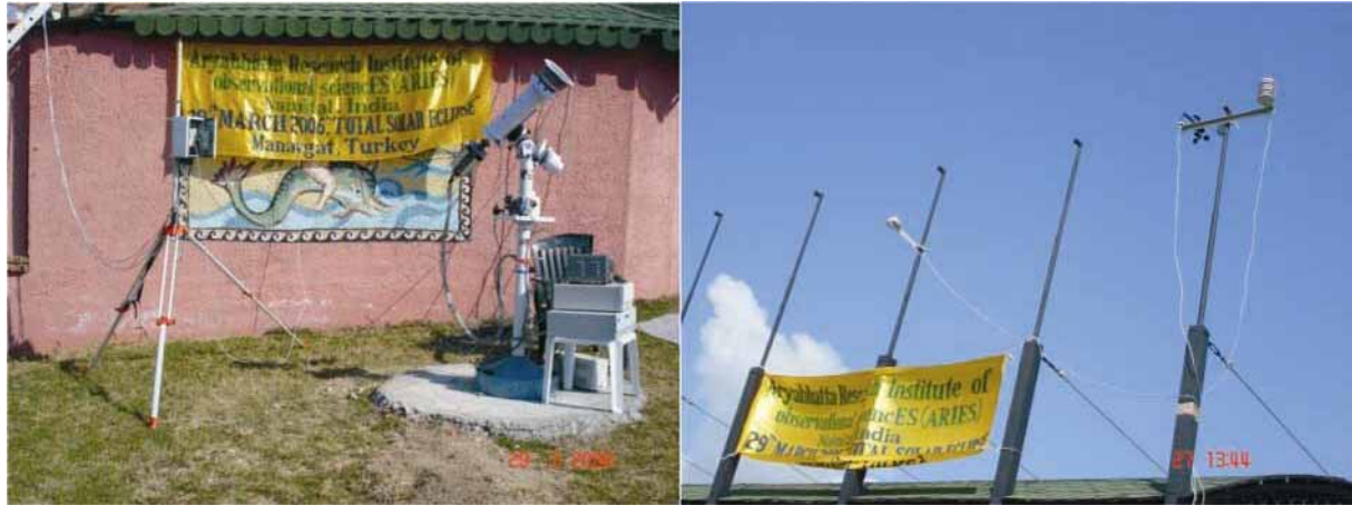
Figure 2. Photograph shows our experimental set-up. (Left panel) Telescope used to make observations of the solar eclipse. The data logger for the mini weather station placed on a tripod is also shown. (Right panel) Different sensors of the mini weather station.
