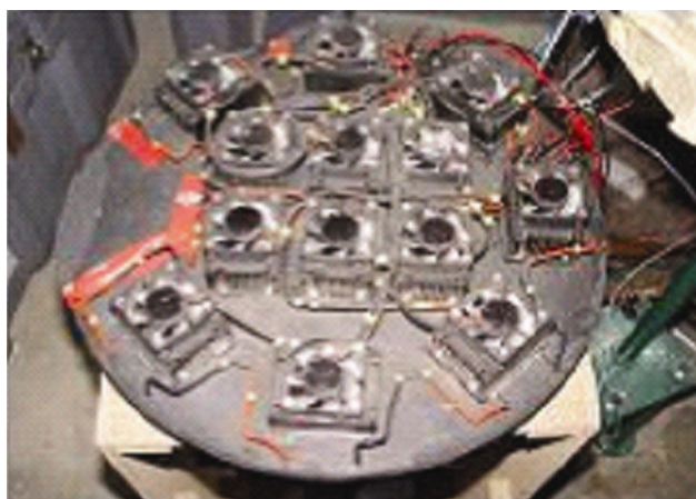
Fig. 3 — Peltier arrangement on filter chamber
