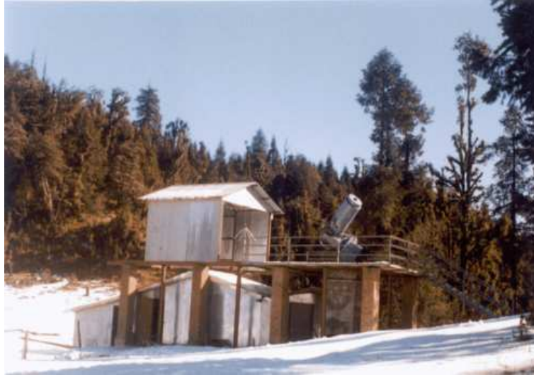
Figure 8. A view of 52-cm telescope installed at Devasthal for seeing and atmospheric extinction measurements
