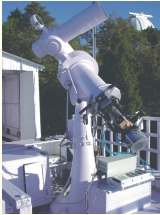
15-cm Coude Solar Tower Telescope equipped with Bernhard Halle H filter & fast CCD Camera for solar activity observations.
