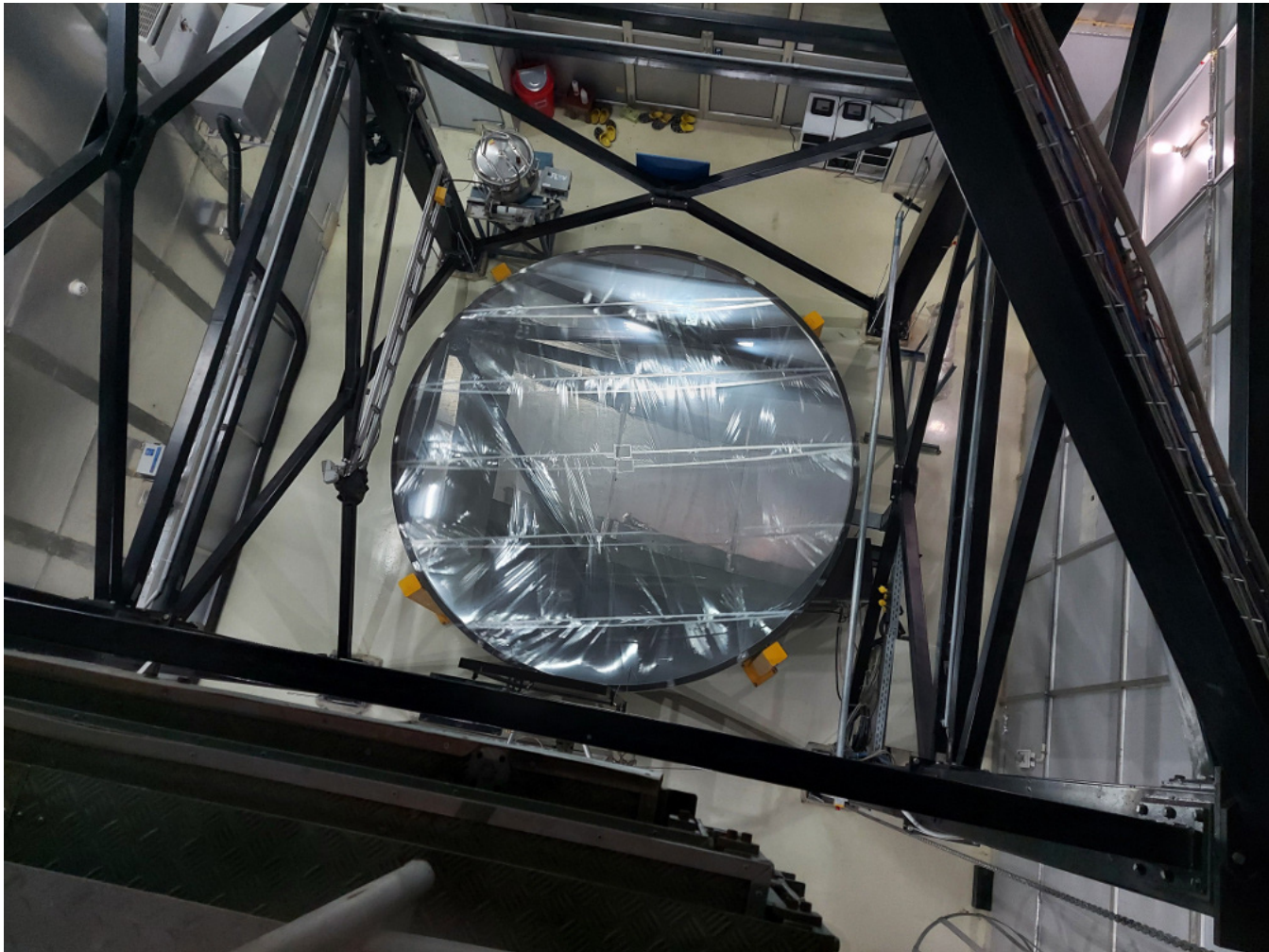
Fig. 5. Top view of the newly formed ILMT mirror. The adhesive tapes of the installed mylar cover are visible over the mirror.
