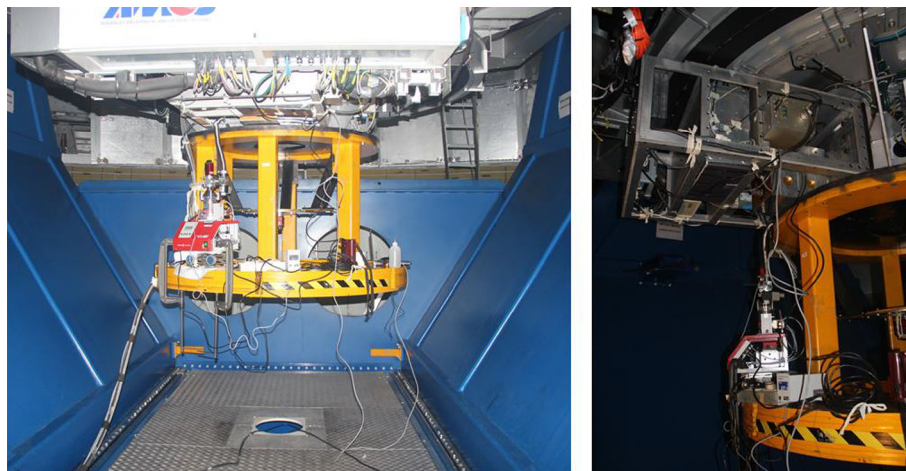
Figure 14. Evacuation setup of the TIRCAM2 camera at the telescope floor after mounting the camera on the side port.
