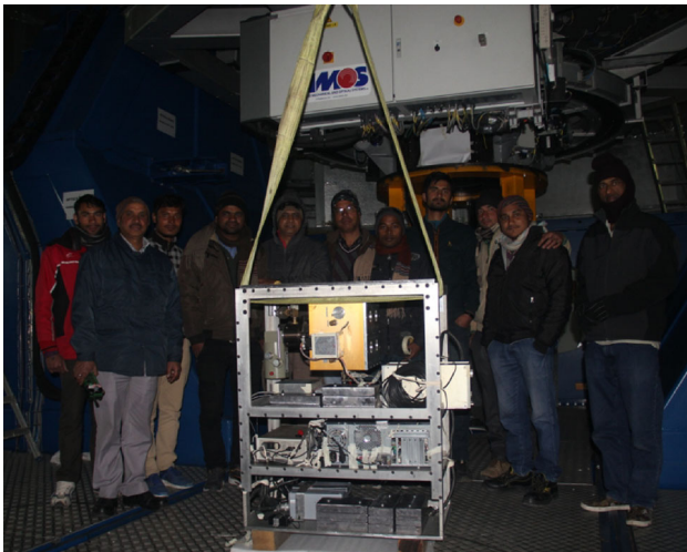
Figure 13. Complete 248 kg TIRCAM2 assembly lifted by the overhead crane during the mounting on the side port.
