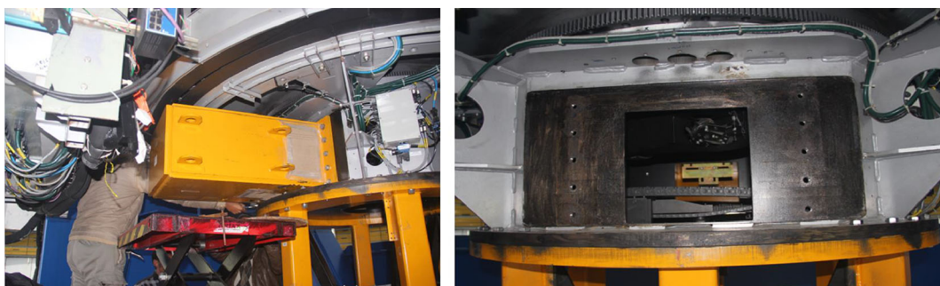
Figure 5. DOT side port with dummy cover (left) and without dummy cover (right).
