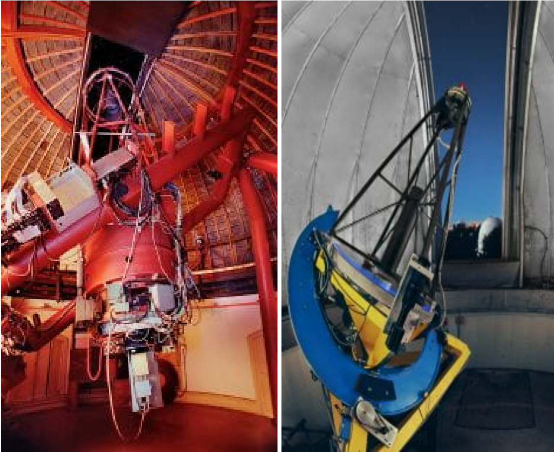
Figure 2.4: Left : The 1 m Nickel telescope at the Lick observatory. Image credit: 1 m Nickel ; Right : The 0.76 m KAIT at the Lick observatory. Image credit: 0.76 m KAIT .
