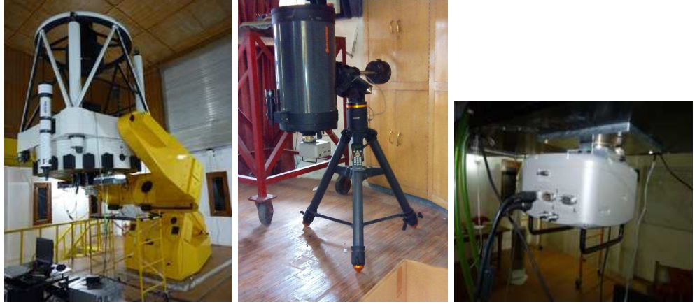
Figure 6.15: TDI set-up at the 1.3m DFOT and C-14" telescopes. From left to right: SBIG camera installed at the focal plane of both telescopes and zoomed image of the SBIG CCD at the DFOT.
