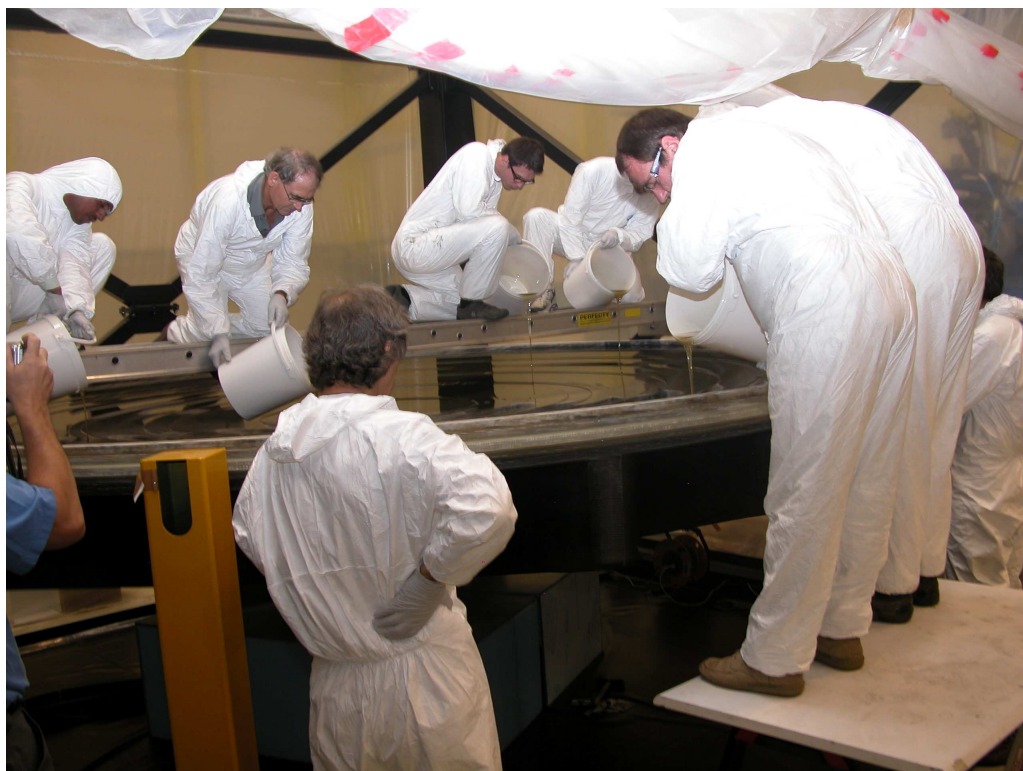
Figure 6.6: Pouring of the PU over the surface of the container. Each of the six sectors were poured at the same time with the continuously rotating container.
