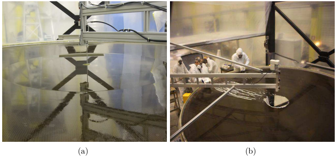
Figure 6.10: Panel (a) Testing and cleaning the container with water. Panel (b) Pouring mercury into the container. The shining mercury can be seen in the central part of the dish.
