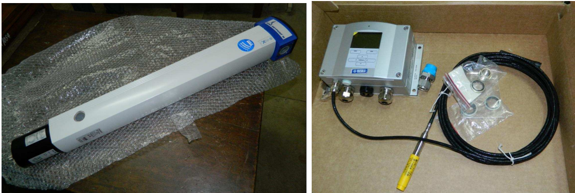
Figure 5.11: Air membrane dryer (left panel) and dew point sensor (right panel)
