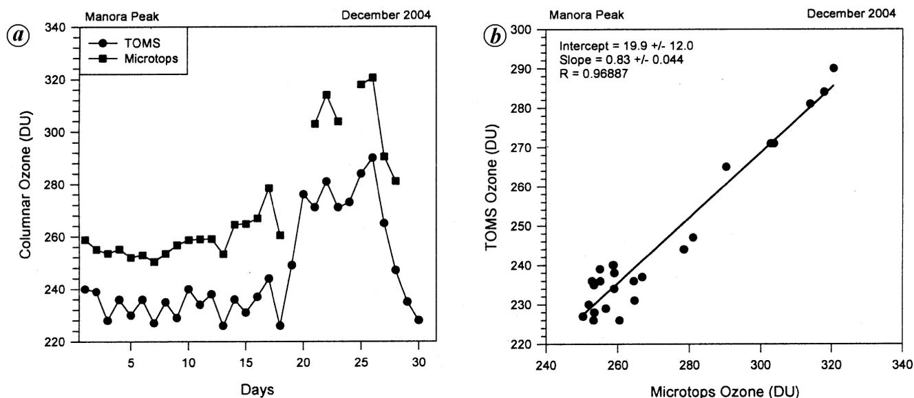
**Figure 4.** (a) Temporal variation of ozone obtained from Microtops II and TOMS and (b) Inter-comparison of ozone obtained from Microtops II and on-board TOMS data.
